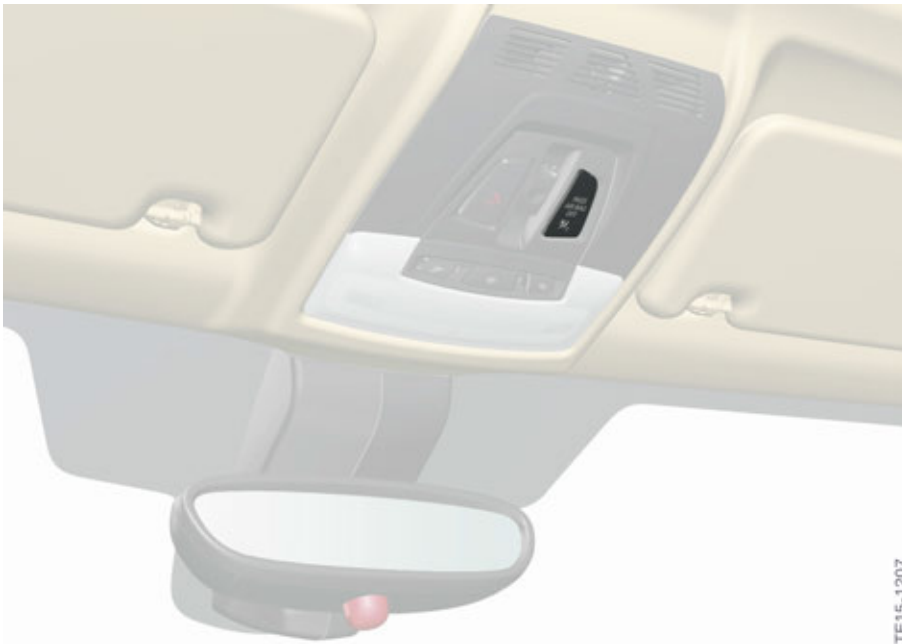
F48 roof function center with indicator lamp for front passenger airbag deactivation in US version
